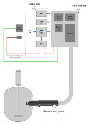
Figure 4. Layout and connection diagram of the measurement system
